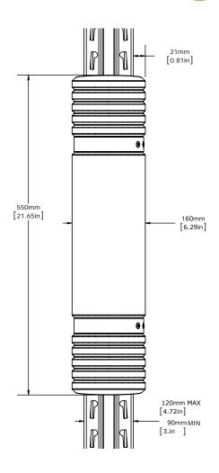
Rack Mounted Guard Kit RACK-GARD-120RM-YEL Materials: Polyethylene body, hook & loop straps
